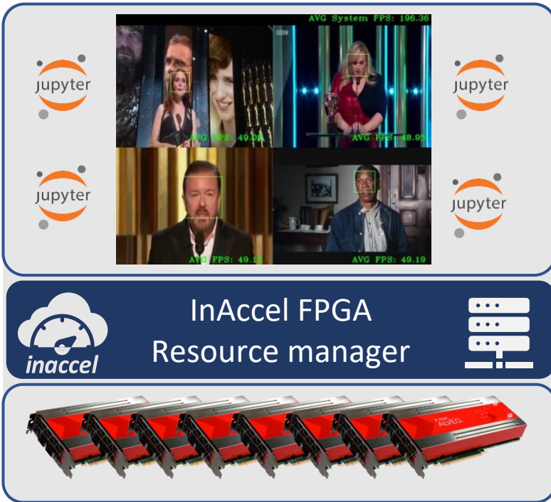
Figure 1. Scalable deployment of Face Detection on a cluster of Alveo U200 FPGA cards using InAccel orchestrator, Click Here and Here to see the relevant videos
